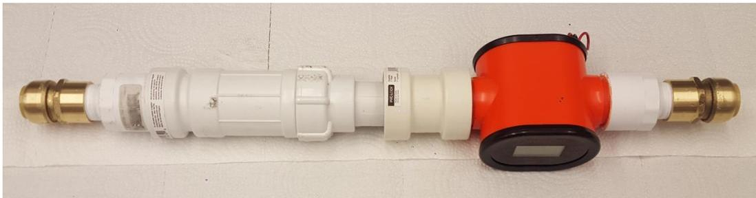
Use a wrench to tightly turn the brass fittings on to the ends of the adapters. These glueless brass fittings attach directly to the  $\frac{3}{4}$ " copper pipe. The extended length of the assembly is  $22 \frac{3}{4}$ " and when compressed is 20". **PLEASE** ensure your backflow preventer has the proper length to accommodate the flow meter assembly.
